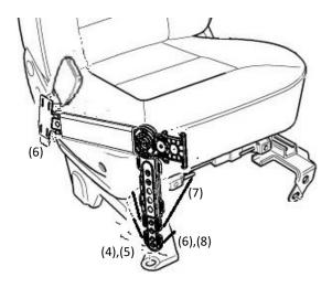
STEP 6: Make final adjustments to Multi-Mount for seat height and length. Multi-Mount should be sticking out past edge of seat approximately 2". Secure Multi-Mount to underneath seat, legs, or track with the Elastic Hook Cords (7). Optional Tie Wrap (8) or 11" Cinch Strap (6) to anchor (4) or (5) to seat leg or pedestal. Some additional Elastic Hook Cords may be required for some vehicle seats.
