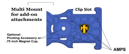
The AMPS hole pattern is an industry standard hole configuration. It consists of four (4) holes located in a rectangular pattern spaced at 1.188" by 1.813" (30mm by 38mm).
