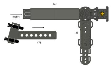
**STEP 3:** Insert Strap Mount (2) into Mounting Rail (1) and set to desired length of seat and gap space to provide the best position (adjusts between 16" and 21"). Adjust length and height by pressing button on Mounting Rail and Support Strut (3), then press the button(s) indicated by the arrows.
